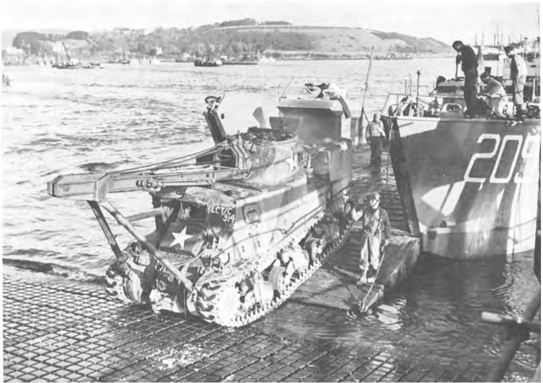
WATERPROOFED TANK RECOVERY VEHICLE moving from a "hard" onto a landing craft.
