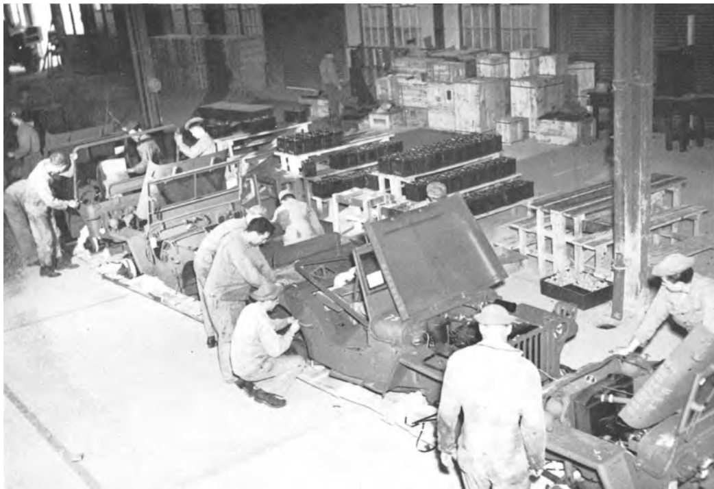
JEEP ASSEMBLY LINE at an ordnance depot, September 1943.
