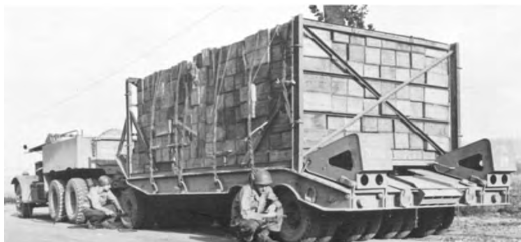
TRACTOR-TRAILER COMBINATIONS used on the Continent: 4-5-ton, 4 x 4, truck tractor, COE, with 2,000-gallon gasoline semitrailer, top; 1½-ton, 4 x 4, truck tractor with 3½-ton stake and platform semitrailer, center; 12-ton, 6 x 4, truck with 45-ton trailer (tank transporter), bottom.
